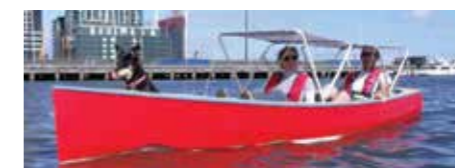
The 5.8m Ostlind pedal boat, Ripple, is built of plywood with twin Hobie Mirage drives.
