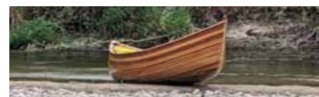
Quasar, a 5.2m wood strip white water canoe, has thigh straps, spins on a dime and surfs well.
