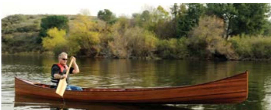
This 5.5m 2024 touring canoe is traditional in style with glassfibre skin and optional ribs.
