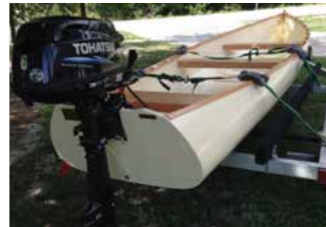
The 4.9m Chickenfeed is a Robb White sport cargo canoe of 2013, powered by a small outboard.
