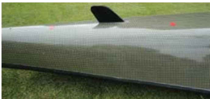
The Marlin with fixed fin rudder.
