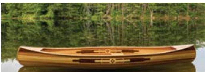
This 3.6m Friedel Otter is built of three colours of cedar and skinned inside and out with glassfibre.
