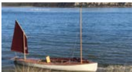
Fry is a 5.2m CLC Waterlust sailing canoe with Hobie auxiliary pedal power.
