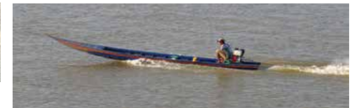
A 6.1m Mekong long tail canoe driven by a small petrol engine.
