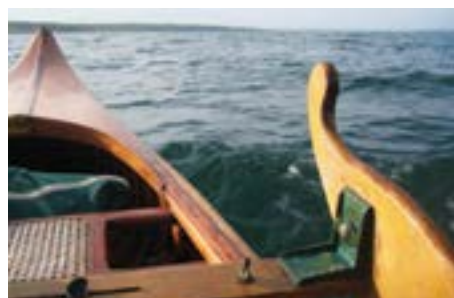
A 5.5m Otca model, built by Old Town in 1930, with lateen rig, having a longer forward deck than usual.
