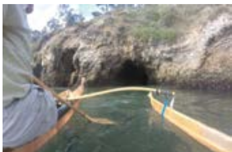
A 3.7m skin on frame ultra lightweight Hawaiian outrigger concept.
