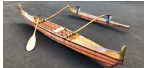
A 3.7m skin on frame ultra lightweight Hawaiian outrigger concept.
