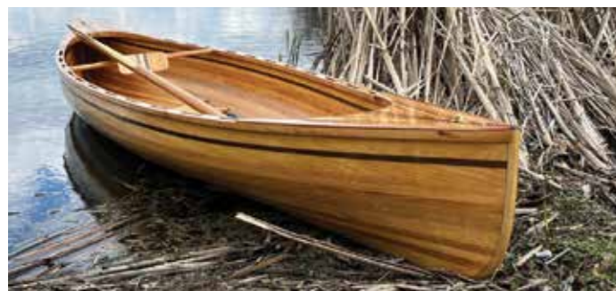
Wee Lassie, a 3m cedar strip canoe built last year to a design inspired by Rushton's 1890s models.
