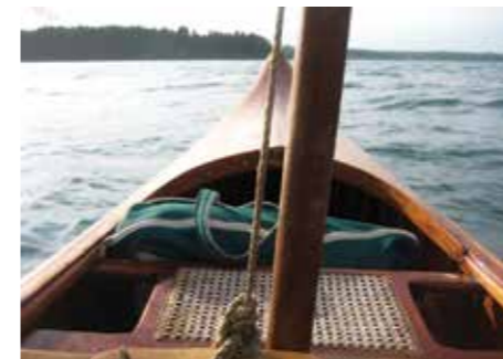
A 5.5m Otca model, built by Old Town in 1930, with lateen rig, having a longer forward deck than usual.
