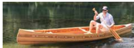
Wayne Timmo's Haereere is a Bob's Special built in 2018 in cedar strip but incorporating decoration using North American cedar and such New Zealand timbers as miro, rimu and rewarewa which were harvested over a century ago.
