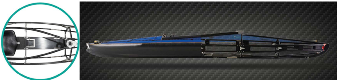
The term 'lath and canvas' for folding kayaks is well out of date. Klepper's Marlin is a 3.8m folding kayak that weighs 20kg and packs into two small bags. Its frame is of carbon fibre which helps it retain its shape and to resist rough handling. Gone are the days of aluminium tubing corroded by seawater.
