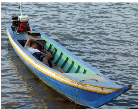
A 6.1m Mekong long tail canoe driven by a small petrol engine.
