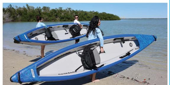
The Sea Eagle Razorlite is the world's only inflatable kayak using drop stitch technology. The floor and two rigid inflatable side walls mean tracking is good and there are adjustable footrests, tie down points and a central lifting point for easy carriage.
