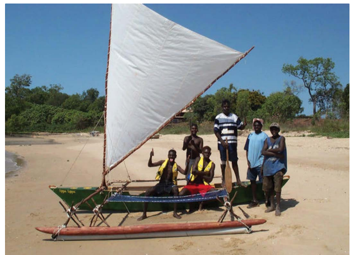
Wharram designed Melanesia outrigger canoe, built from 2 sheets of ply.
