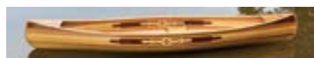
This 3.6m Friedel Otter is built of three colours of cedar and skinned inside and out with glassfibre.
