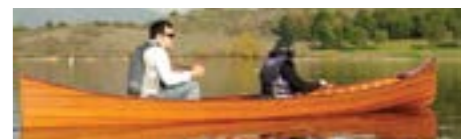
This 5.5m 2024 touring canoe is traditional in style with glassfibre skin and optional ribs.
