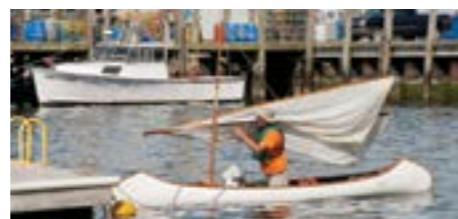
This 1900 Kingsbury canoe has a lateen sailing rig.
