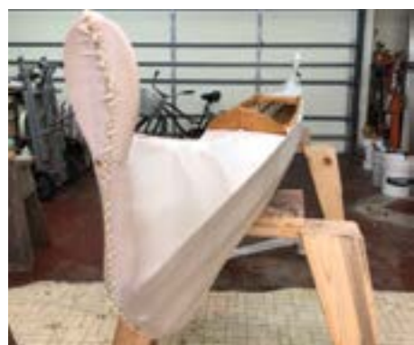
A 3.7m skin on frame ultra lightweight Hawaiian outrigger concept.
