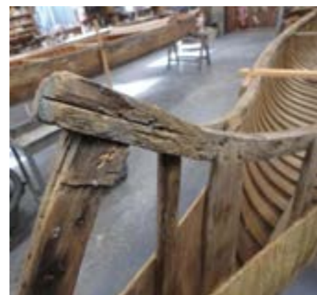
Thought to be a 1901 model by the company that would become Old Town, the bow and stern lashings are similar to those of a birchbark canoe.
