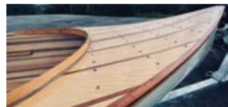
Gator Won is a cedar strip 5.5m freighter with a powerful Mercury outboard.
