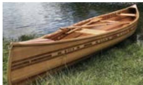
Wayne Timmo's Haereere is a Bob's Special built in 2018 in cedar strip but incorporating decoration using North American cedar and such New Zealand timbers as miro, rimu and rewarewa which were harvested over a century ago.
