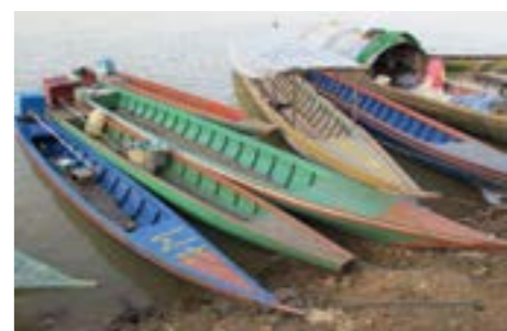
These 6.1m Mekong long tail canoes are driven by small petrol engines.
